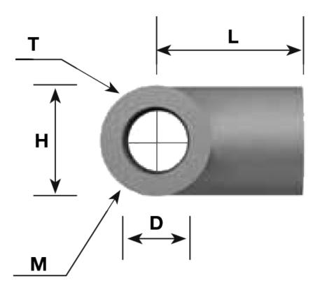
D =  $\emptyset 10,1$ H = 18 L = 24 M = Metal T (Thickness) = 18
